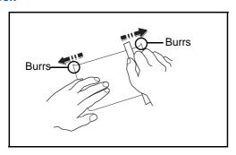
Before loading Hagaki into the multi purpose tray, fan them and align the edges. If the Hagaki paper is curled, straighten it before loading. Printing onto curled Hagaki may cause jams.
